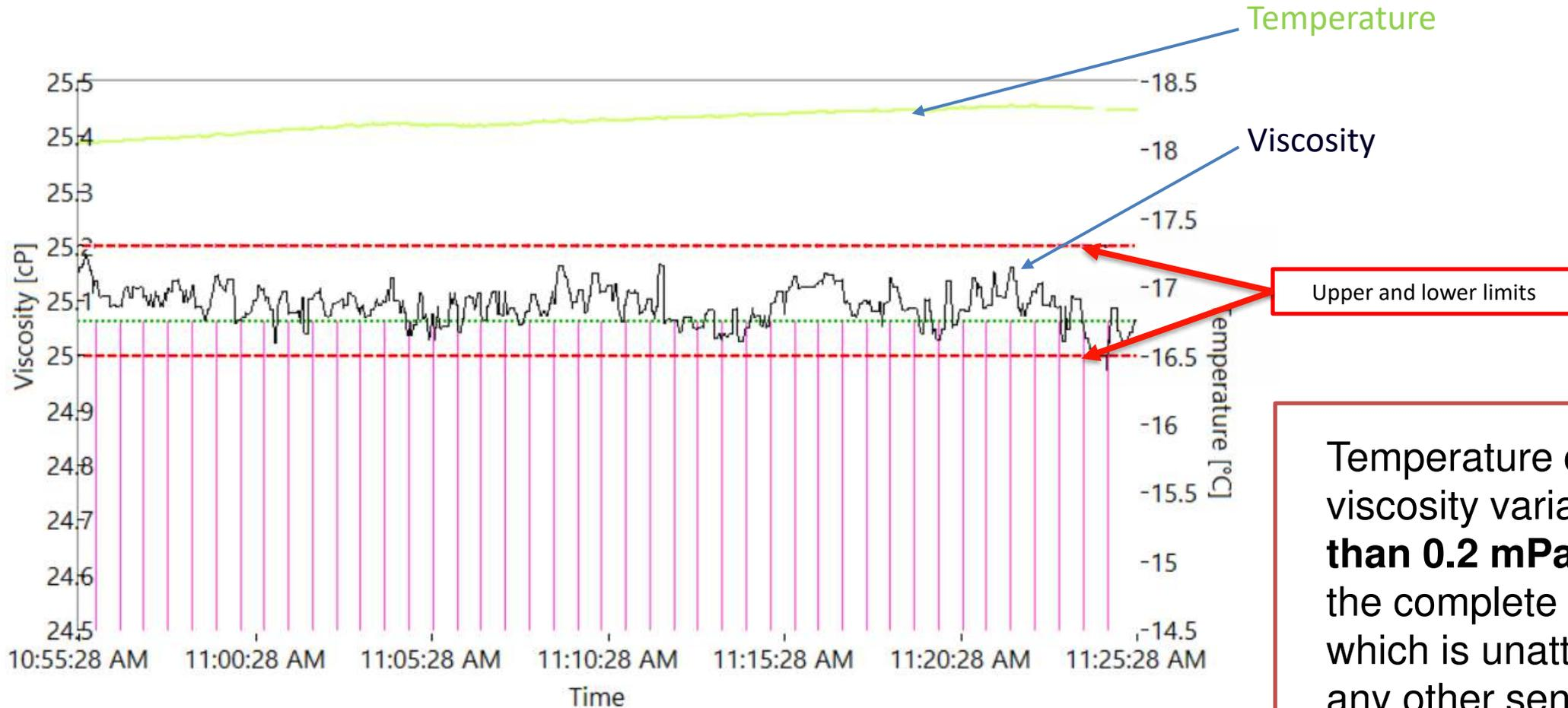
Temperature compensated viscosity variation is **less than 0.2 mPaS** throughout the complete print run; which is unattainable with any other sensor or traditional instruments.
