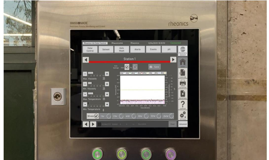
InkSight predictive tracking controller installed on machine
