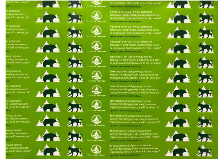
(a) dE2000 for a run of 24,500 meters spread over 5 days and 13 reels (b) sample of print
