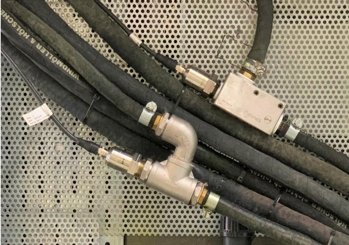
Two SRV inline viscometers installed on the ink hoses from pump to the doctor chamber
