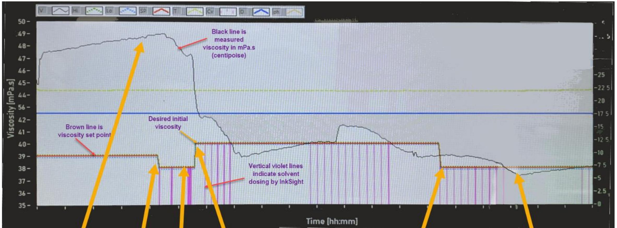
Initial ink viscosity about 48 cPs; desired working viscosity ca. 40 cPs. Dilution is needed
